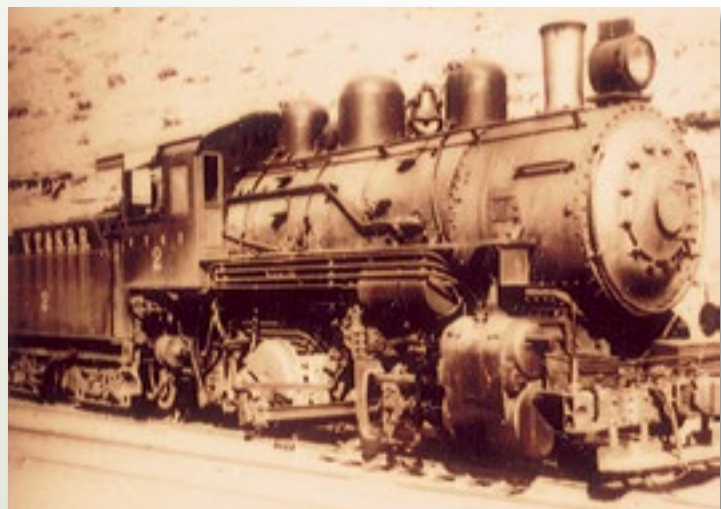
Climax engine used to build track from Jerome to Clarkdale
